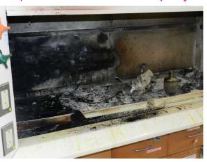
Accidental mixing of incompatible chemicals causes lab explosions! The photo above resulted from mixing incompatible laboratory waste.
