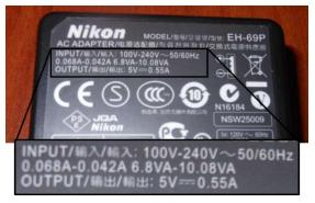
This Nikon AC Adapter is used to charge a camera. It has several interesting pieces of information on it. The range of voltages (100V-240V) means it will work in a variety of countries (in the US power is supplied at 120V). It also gives a range of amps and a range of numbers labeled VA. The VA numbers are volt amps (or watts). At a maximum this plug will require 10.08W.
