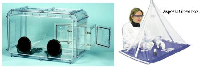
Glove boxes are used when extreme containment is needed for Biological and highly toxic chemicals, especially for substances that can be swept out of containers by the airflow in hoods.
