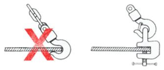
The pictures show improper hooking methods, which may cause the hook to elongate or bend. These hooking methods may also obstruct the load chain flow to the load sheave and prevent the lever hoist from operating properly.
